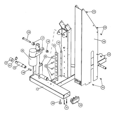
3. If you removed the lift axle wear tube because you are installing a new lower lift shaft (as described in Procedure 7.10), visually inspect the lift axle wear tube. If the wear tube is worn or defective . . .
